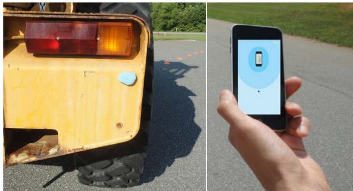
**FIGURE 8 Bluetooth proximity detection and alert system—beacon mounted on a wheel loader (left), and personal protection unit held by a test person (right).**
